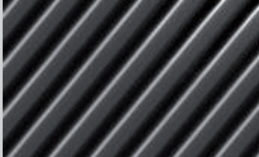
diffractive grating (6µm pitch) (© Centro Ricerche FIAT)
